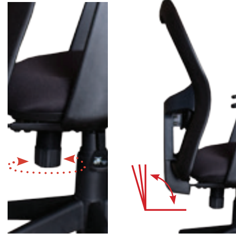
Adjustable Tilt Tension Twist knob under seat to adjust backrest tension. Twisting clockwise increases tension.
